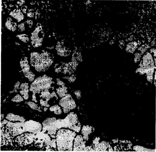
A black and white micrograph showing a grain structure with dark, irregularly shaped regions of graphite segregated along the grain boundaries. The grains themselves are lighter and have a somewhat granular texture. | Выделение графита в виде сегрегаций, а также по границам зерен | 4                        |
